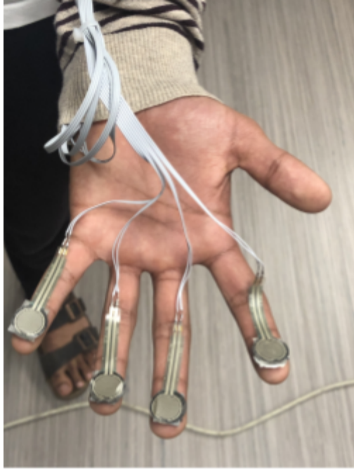
Figure 7: FSR Only on User's Hand
